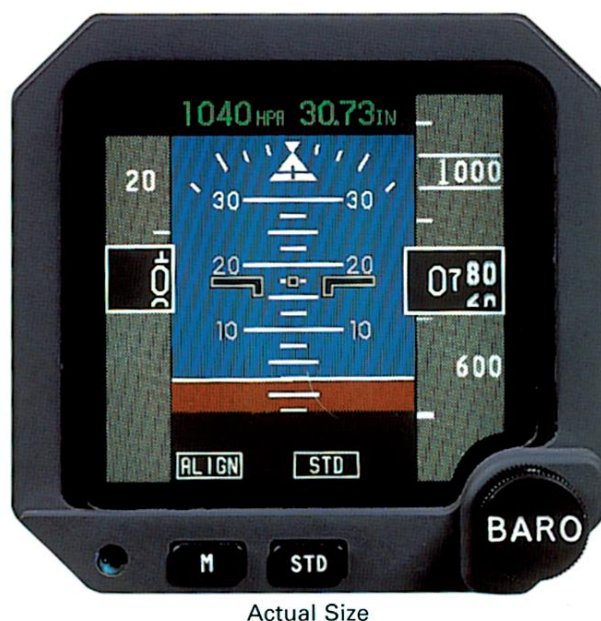
Fig. 4 – Standby Instrument System (Ref. 4)
